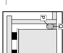
To realize the potential of some production machinery, it is necessary to create an isolated environment that performs a dual function of absorbing the machine's own work-generated energy while preventing transmissions of ambient vibration to the machine itself. The inertia block provides mass to assure the optimum performance of the isolation material and the rigid anchoring base required for the permanent alignment of the machine being installed.
